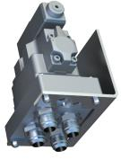
Mounted in the operator's preferred position directly to the host machine. Externally mounted 2 Way Valves take the one way flow from your hammer circuit and then utilising an electrical switch (runs back to the cab), allows for easy forward and reverse control of the drive unit.
